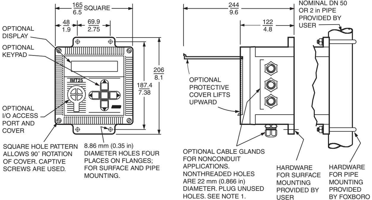
**SURFACE AND PIPE MOUNTED TRANSMITTER - OPTIONAL DUAL COMPARTMENT**
