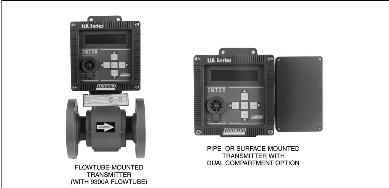
The IMT25 Magnetic Flow Transmitter, together with an 8000A Wafer Body, or 2800, 8300, 9100A, 9200A, or 9300A Flanged Body Flowtube, combines to form a Magnetic Flowmeter with pulsed dc excitation.
