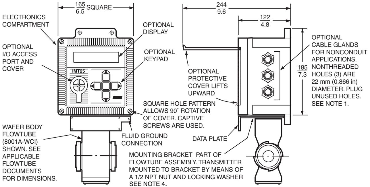
**FLOWTUBE MOUNTED TRANSMITTER - OPTIONAL DUAL COMPARTMENT**
